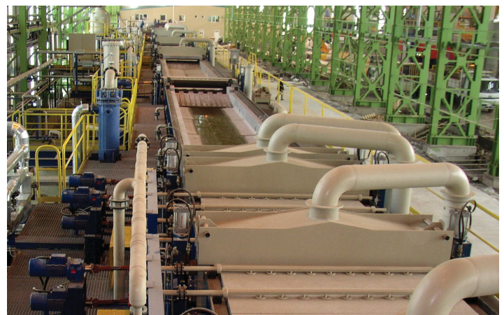
Fig 3 Turbulent shallow tank for pickling with HCl
